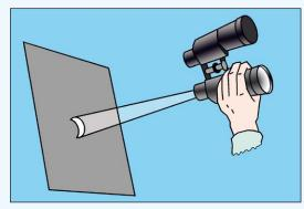
A pair of binoculars can stand in for a pinhole. Cover one eyepiece with the lens cap, then when the binoculars are pointed at the Sun you should see its image projected onto the plain card. Use the focus wheel to sharpen the image. This method works best if both the card and binoculars are mounted on a tripod.
