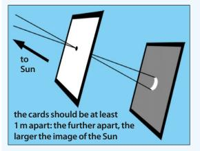
A simple yet safe way to view the solar eclipse is by making a pinhole viewer.
